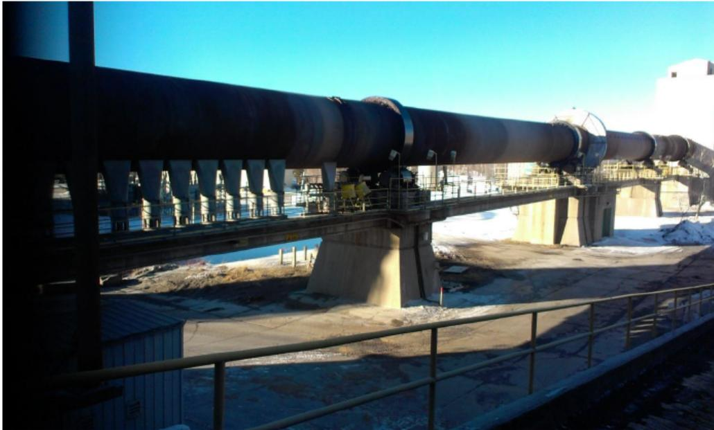
**Figure 1:** Image of the rotary cement kiln at Lafarge Inc, Brookfield [3]
