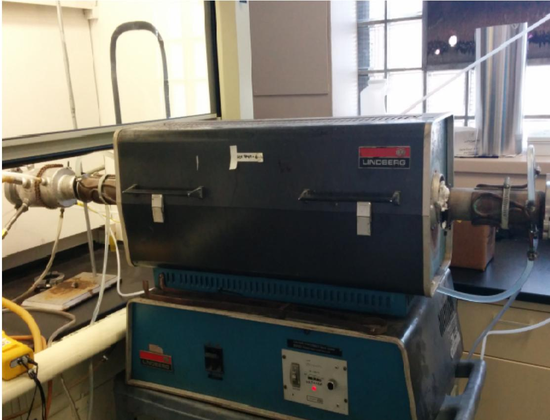
**Figure 3:** The Electric tube furnace used for combustion studies
